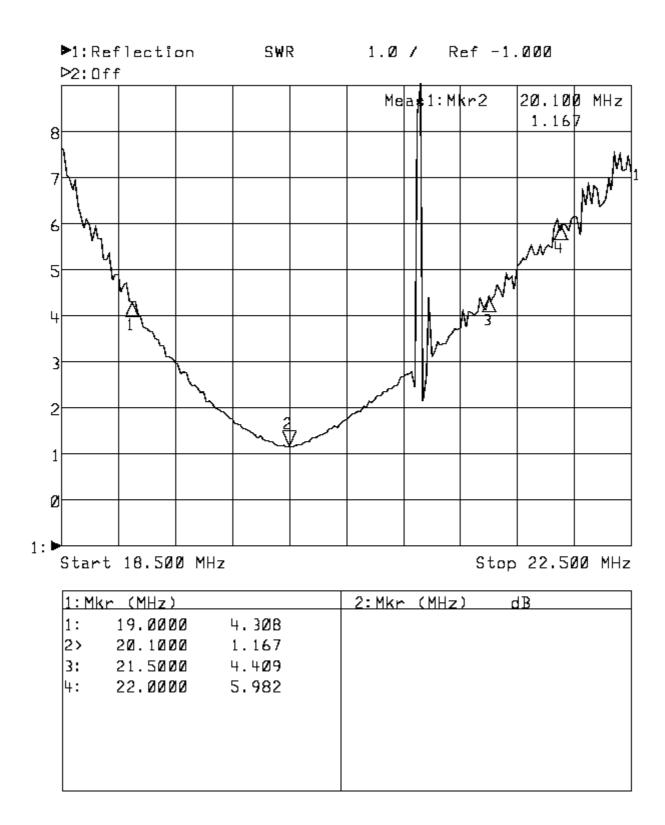
The sudden rise in VSWR at ~21MHz is because of the LO leakage at RF port.
